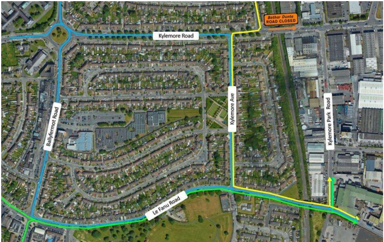
Figure 5-57 Kylemore Southbound Traffic Diversions – Light Vehicles
