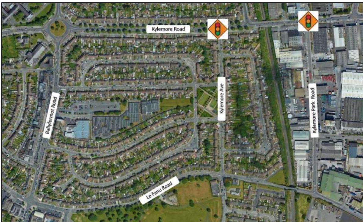
Figure 5-49 Temporary Traffic Signal Locations
