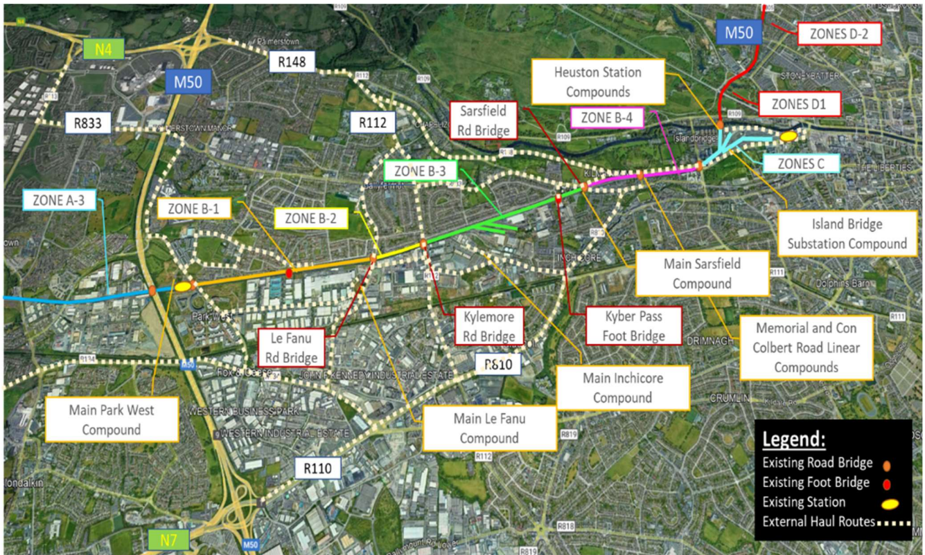
Figure 5-53 Sub-Zone B-1: External Haul Routes
